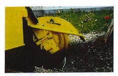
SWING ARC. The sweep arc measures 103" (261.6 cm). The below-ground cutting depth of 25" (63.5 cm) allows operators to cut even the largest stumps efficiently. The rear deck design allows for chip containment capacity of approximately 68 cu ft (1.9 cu/m).
